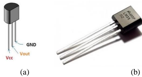
Figure 2: (a) Lm35 pinout (b) Lm35 sensor
